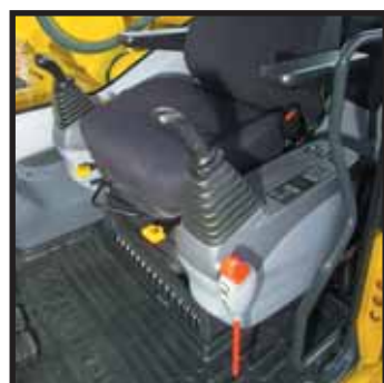
Seat sliding range: 340 mm
