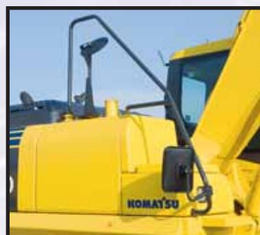
Large handrail for safe access
