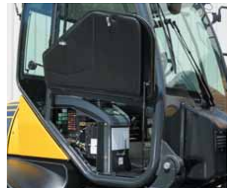
Side cover for quick maintenance access
