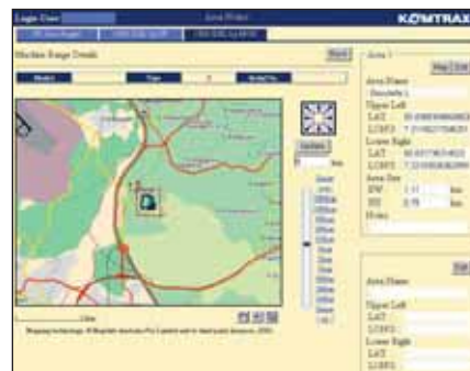
Added security - The "engine lock" feature allows to program when a machine's engine can be started. And with "geo-fence", KOMTRAX™ sends notification every time your machine moves in or out of a predetermined operating area.
