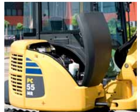
Front bonnet: fuel tank refilling
